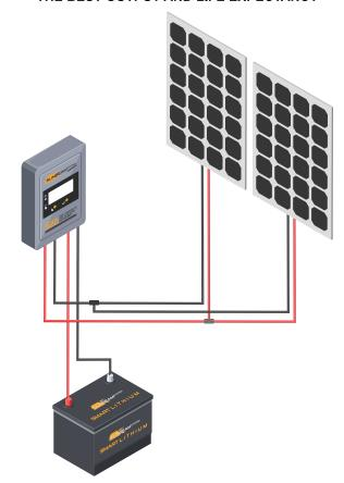
FOR 24V & 48V SYSTEMS IT IS COMMON TO PUT THE SOLAR PANELS IN SERIES BUT WE RECOMMEND THE USE OF A "BOOST" CHARGE CONTROLLER WHICH ALLOWS A PARALLEL INSTALLATION.
